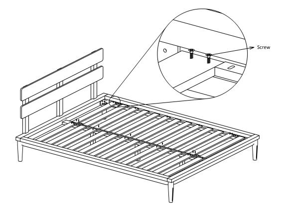
i) Now fix screw at 1st,3rd,6th,9th and 12th slates as shown in fig. (1st and 12th slate are fixed with two screws and remaining are fixed by single screw.)
