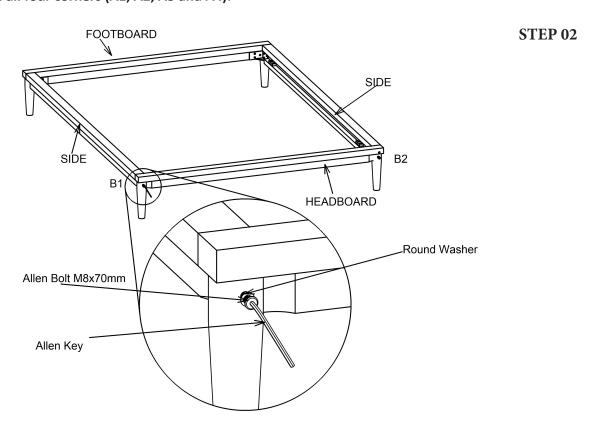
i) Insert round washer then loosely tighten M8 x 70mm Allen bolt to the backside of the headboard with the Allen key (B1 and B2).
