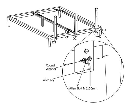
i) Attach Part A (headboard support) by inserting a round washer then loosely tighten with Allen bolt M8 x 50mm using the Allen key(D1, D2 and D3).
