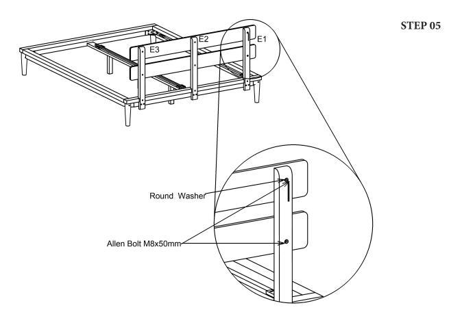
i) Attach Part B (headboard) to each of the Part A (headboard support) pieces by inserting a Round washer and Allen bolt M8 x 50mm loosely tighten with an Allen key (E1, E2 and E3).NOW, FULLY TIGHTEN ALL THE ALLEN BOLT USING ALLEN KEY.
